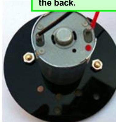
Fix the acrylic to the pillar using screws, but not overexertion to avoid broken due to the thin acrylic.
