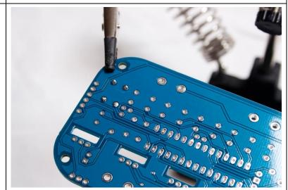
Next you can solder the rest of the resistors in place. R2 and R3 are 150  $\Omega$ , and R4 is 1.5 k $\Omega$ .
