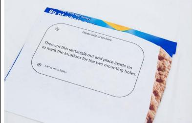
Insert the cardboard/drilling guide into the tin as shown. Place the PCB on a block of hardwood and drill the two mounting holes through the tin with a 1/8" (or 3 mm) drill bit. Begin drilling slowly to keep the drill bit centered on the marks. It's okay if the tin gets deformed slightly around the holes.
