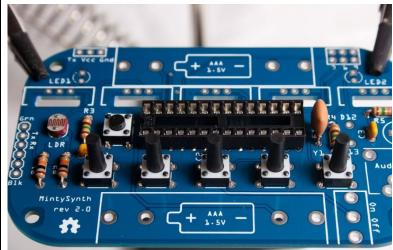
Now let's add the electrolytic capacitor, C4. This one *is* polarized, so be sure that the gray band on the side of the capacitor points to the edge of the PCB, as shown.
