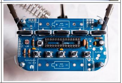
The small plate to which each thumbwheel is mounted should extend into the slot in the cover plate, held firmly against the back of the slot by the pin.
