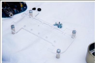
Now position the cover plate over the buttons and wheels. Gently guide each thumbwheel so the small pin that you bent upward engages into the tiny hole in the acrylic. You will gradually be able to lower the cover plate down until the standoffs are almost touching the PCB. Don't force the cover plate down if it won't go—it probably means that one of the pins isn't engaged correctly.
