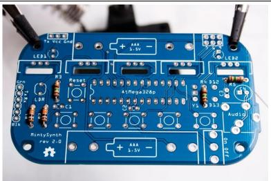
Next we'll add the small yellow ceramic capacitors, C1, C2, and C3. These are all the same, so you don't need to worry about the value. There's also no polarity, so they can go either way. Try to make sure that they are fully seated in the PCB, and sitting vertically. You can bend out the leads on the back to hold them in place, as you did with the resistors.
