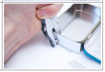
Here's the completed hole. If you prefer to use a drill, a brad-point drill bit is recommended to help minimize deforming the thin metal. Also, it is necessary to put a small block of hardwood under the metal to support it while drilling. Some people recommend filling the tin with water, then freezing it, so the ice will support the metal as you drill.
