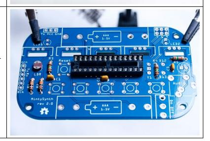
Now add the ceramic oscillator, Y1. Again, there's no polarity, so it can go either way. It helps to have some method of holding it vertical while you solder. Here I've used one of the clips on the helping hand to support it while I solder.
