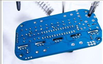
Now add the three headers, with the short ends of the pins in the PCB. These can be a little tricky to hold vertically while you solder, so again use the helping hand where necessary. Solder one or two pins first and check to make sure the header is vertical.
