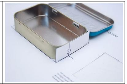
The easiest way to make the ¼" hole for the audio jack is with a paper-hole punch, which typically costs less than \$2. However, the punch may need to be modified to remove the paper guide, as shown, so that it can reach close enough to the bottom of the tin. The guide can often be removed by pulling it out with a pair of pliers. If there's a small tray on the bottom of the punch for collecting "dots", you may have to remove that too (you can usually just pull them off).
