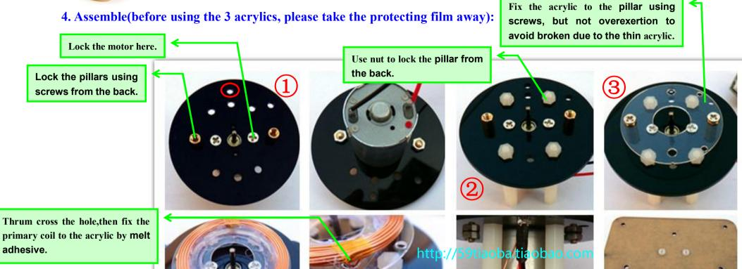
Infrared cross the hole from the back(like step ①,the red circle place).
