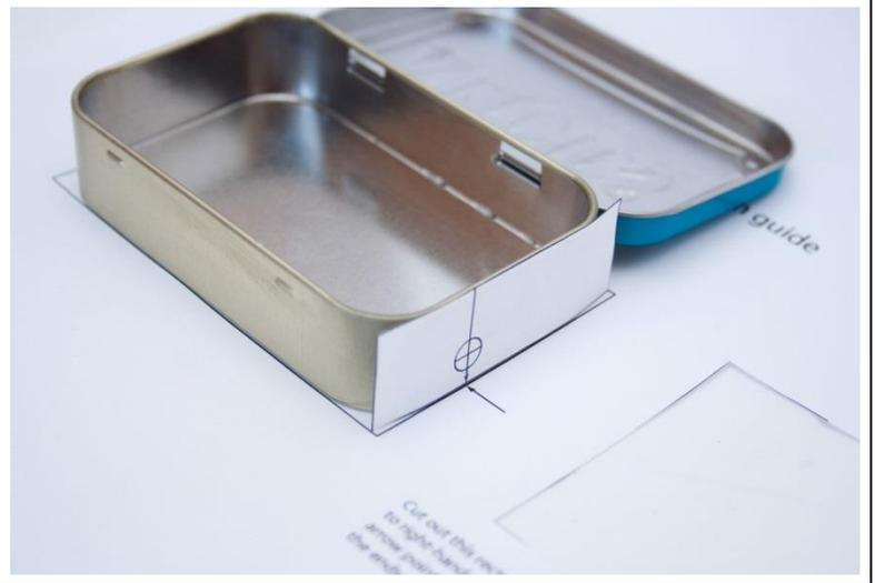
The easiest way to make the  $\frac{1}{4}$ " hole for the audio jack is with a paper-hole punch, which typically costs less than \$2. However, the punch may need to be modified to remove the paper guide, so that it can reach close enough to the bottom of the tin. The guide can often be removed by pulling it out with a pair of pliers. If there's a small tray on the bottom of the punch for collecting "dots", you may have to remove that too (you can usually just pull them off).
